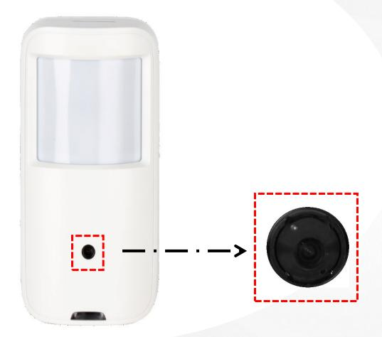
The lens which we choose is an pinhole lens. It is hidden, not easy to found. And the field of view angle is 100 .5° which can cover the detection range of the PIR.
