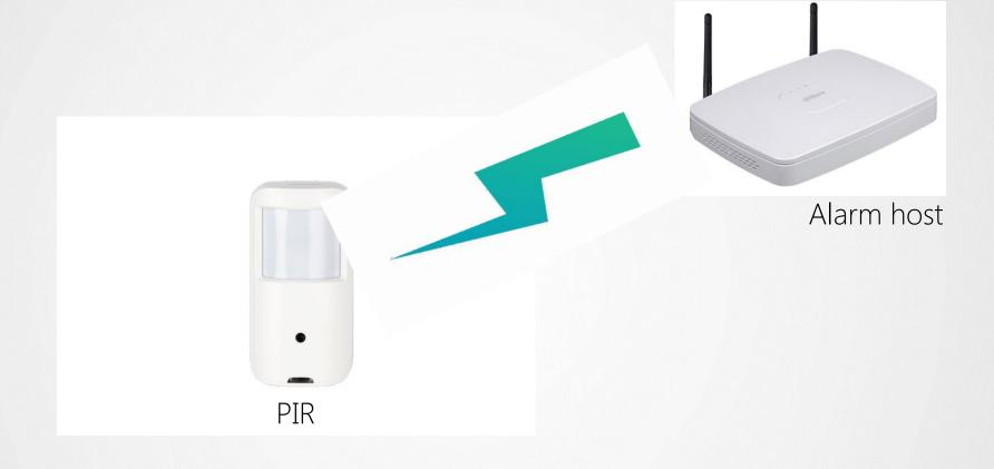
The wireless communication distance is up to 1km in an open environment (only for –W model)
